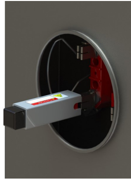
FAIL: Socket jaw has significant loss of spring force
